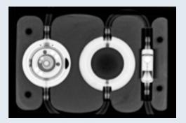
X-ray image of Valve Board with proGAV 2.0 with prechamber, lumbar right (pressure rating of proGAV 2.0 - 20 cmH<sub>2</sub>O pressure rating of SHUNTASSISTANT 2.0 - 25 cmH<sub>2</sub>0)
